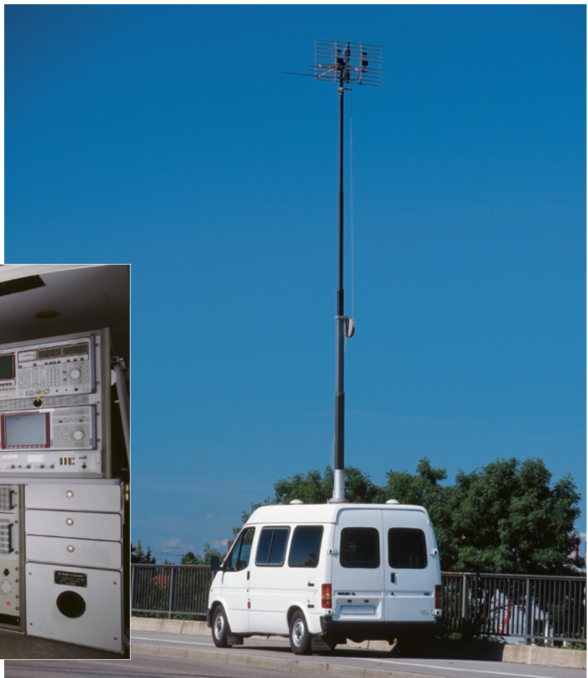
Test vehicle with Coverage Measurement System R&S ARGUS-FMTV
